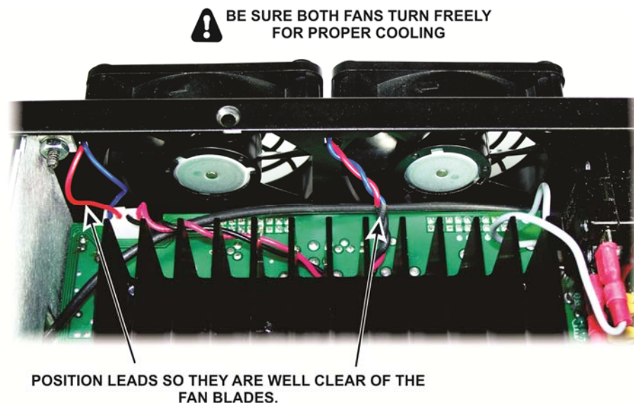
Figure 25. Positioning the Fan Leads.
